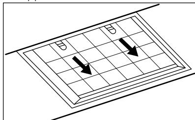
3. Slightly tilt the front of the filter downwards, then pull.
